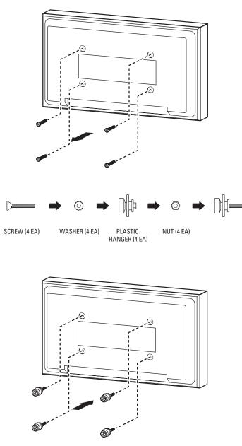
Figure 3. Installing Plastic Holders
